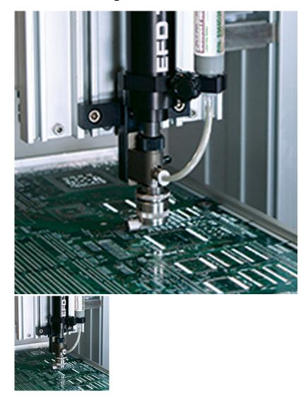
The 794 Series auger valve makes precise, repeatable deposits without damage to the metal alloy particles in fluids such as solder paste and silver epoxies. For highly abrasive fluids such as thermal interface materials (TIM), use the 794-TC Auger Series with tungsten carbide wetted parts.
