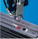
Nordson EFD's unique MicroMark® spray marking systems eliminate clogging, maintenance, and downtime by using a programmable air delay after each cycle to clean the spray nozzle.
