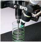
Nordson EFD Radial Spinner Valve System provides an efficient, cost-effective way to apply production fluids inside cylindrical parts between 10.2 mm (0.4") and 127 mm (5") in diameter.
