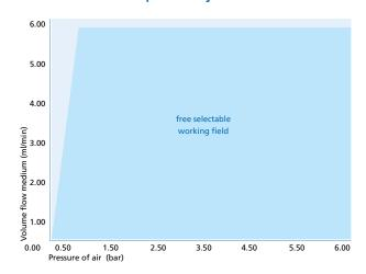
Working field is free selectable. Volume flow of air & medium are <u>independently</u> adjustable.
