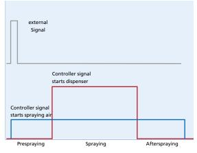
Prespraying, spraying, afterspraying and pressure are customer specifically adjustable. Thereby individual spray contours are possible.
