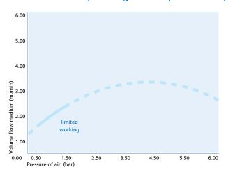
Limited working field. Volume flow of air & medium are interdependent.
