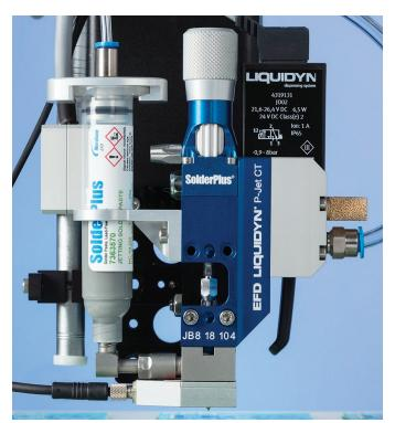
The high-performance Liquidyn P-Jet SolderPlus valve provides a complete solution for non-contact dispensing with solder paste.
